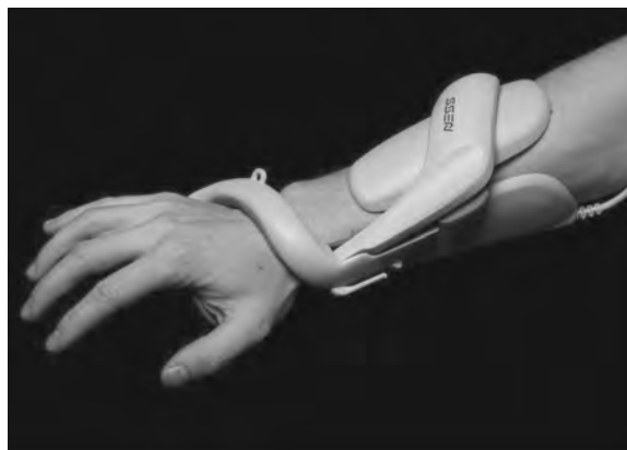
Figure 22.1 A hybrid brace–transcutaneous neuroprosthesis system (NESS H200) that is worn on the hand and forearm. The exoskeleton positions the wrist in a functional position and the five surface electrodes built into the exoskeleton stimulate specific muscles to provide coordinated hand opening and closing. (Courtesy of Bioness Inc., Valencia, CA.)
