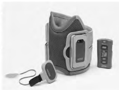
Figure 22.4 Three FDA-approved transcutaneous peroneal nerve stimulators. The Odstock Dropped Foot Stimulator (left-top; courtesy of the Department of Medical Physics and Biomedical Engineering, Salisbury District Hospital, Salisbury, UK) and the wireless L300 (left-bottom; courtesy of Bioness Inc., Valencia, CA) uses a heel switch to trigger ankle dorsiflexion. The WalkAide (right; courtesy of Innovative Neurotronics, Austin, TX) uses a tilt sensor to trigger ankle dorsiflexion.
