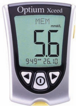
Figure 67 The Optium Xceed meter has the unique ability to measure both blood glucose and blood ketone levels. Not only are these functions useful in hospital patients with diabetic metabolic decompensation, but also they can be very helpful in allowing diabetic patients in the community to detect impending ketosis and thus take corrective action to prevent diabetic ketoacidosis
